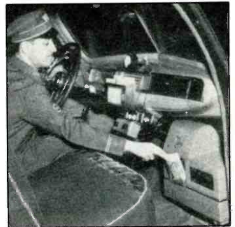
Inside the Western Union "Telecar" was a FAX machine hooked to a VHF two-way radio system. Telegrams could be sent/received, by FAX, directly between the vehicle and the central office.
